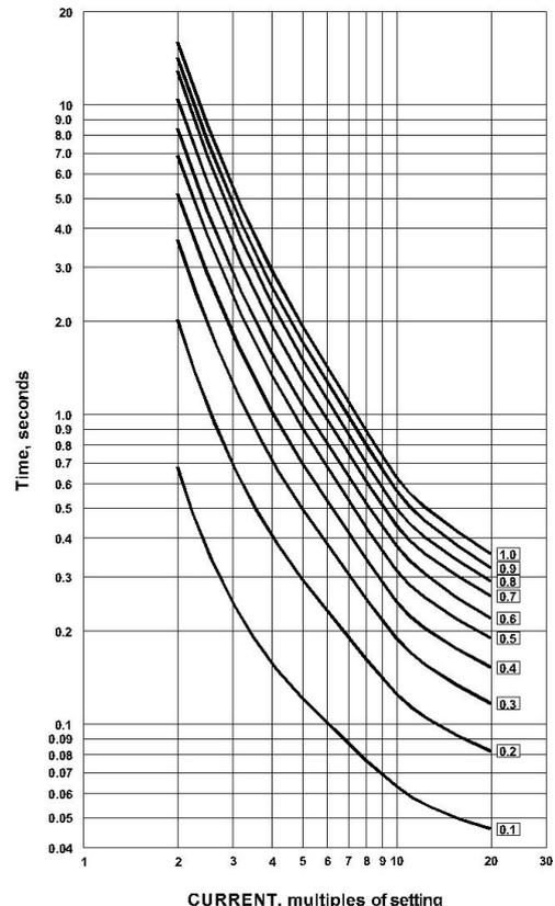
Fig.1 Time / Current Characteristic
